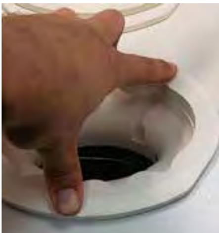
7. Visually inspect the insert and replace if wear or damage are noted.
