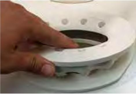
4. Push down on the other side of the insert to seat it against the filter flange.
