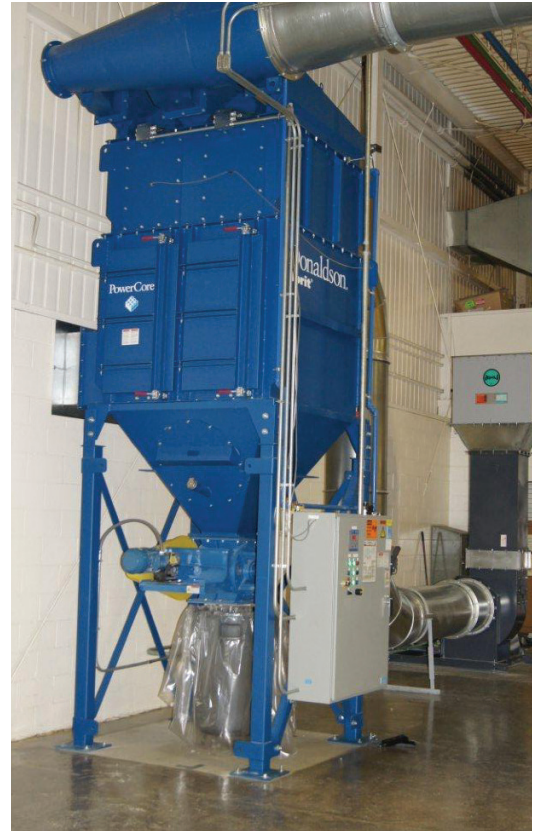
POWERCORE® VL 2-8 on Paper Pleating Process 10,000 cfm (16,987 m 3 /h)
