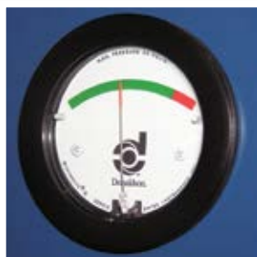
Differential pressure gauge(s) identifies filter maintenance.
