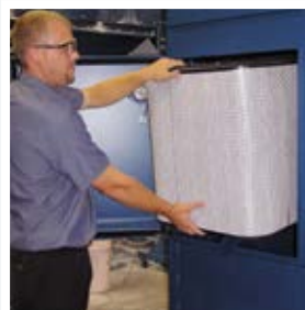
Filter is easily removed.
